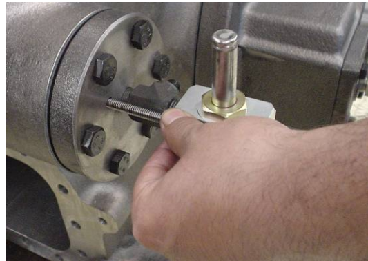
Position adjustment of the unloader push rod
