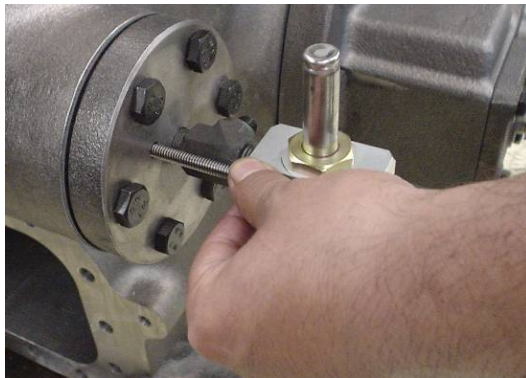
Adjustment of push rod position
